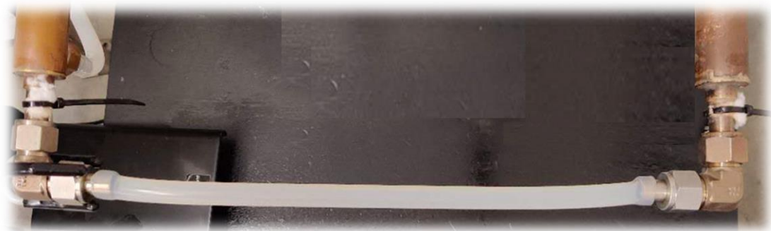
Figure 3-14 Photo of a transparent rubber tube replacing the heating tube
