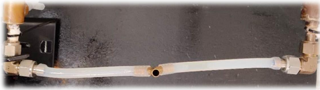
Figure 3-15 Photo of a T-connector installed in the middle of the transparent rubber tube
