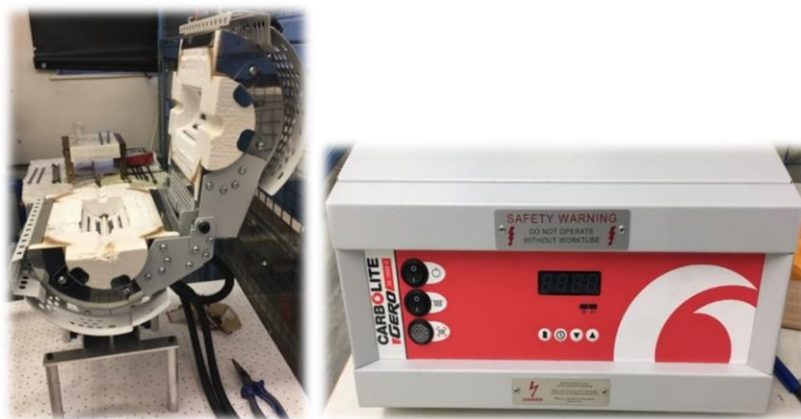
Figure 3-6 Furnace and control panel
