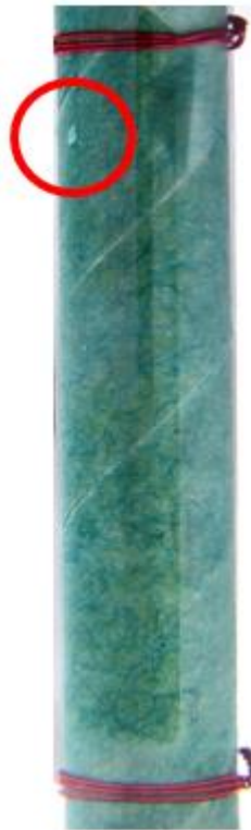
Figure 6-30 – Example of pooling behaviour beginning on 26% relative saturation TUP sample, 26 W test.
