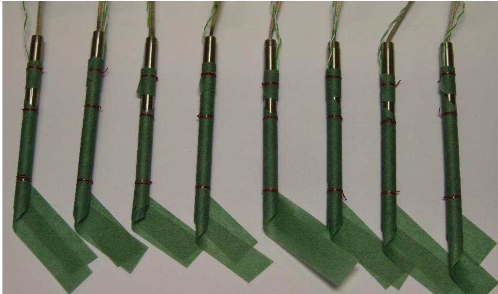
Figure 6-5 – Consistency in construction of wrapping technique of TUP samples.
