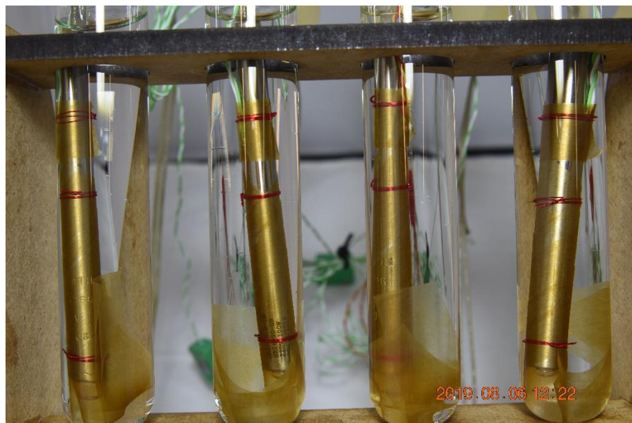
Figure 6-9 – NTUP samples immediately after impregnation with Gemini X, before re-moistening.
