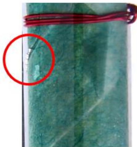
Figure 6-31 – Example of bubbles releasing from overlap of paper insulation on 26% relative saturation TUP sample, 26 W test.
