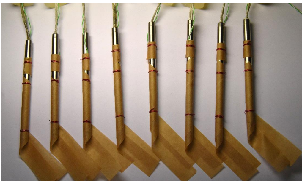
Figure 6-4 – Consistency in construction of wrapping technique of NTUP samples.
