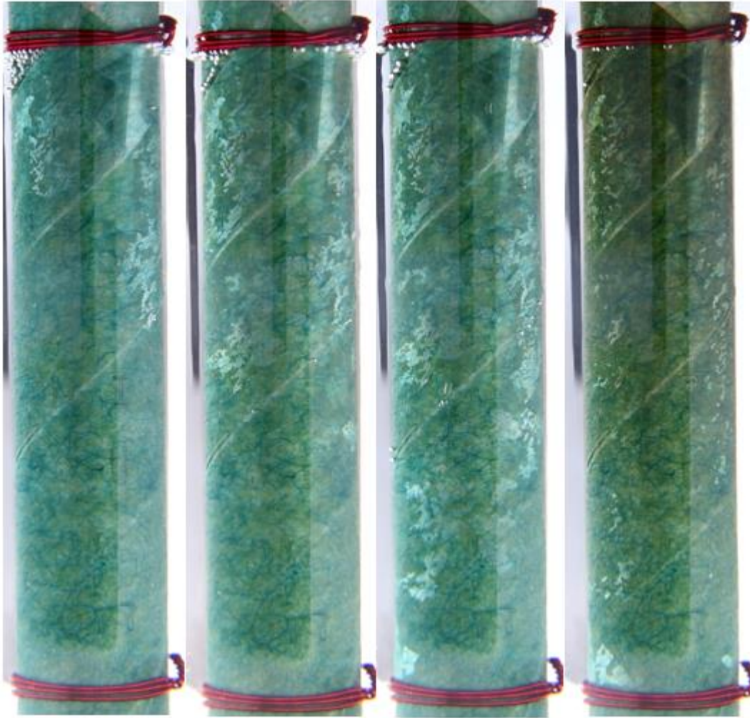
Figure 6-32 – Progression of pooling and bubbling in sample with time for 26% relative saturation TUP sample, 26 W test. Capture at 30 seconds, 3 minutes, 5 minutes and 27.5 minutes after first bubble from left to right.
