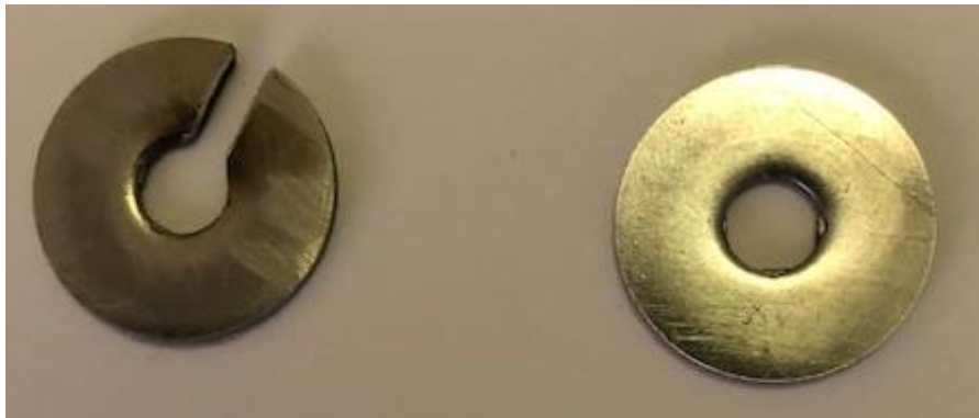
Figure 5-2 – Two styles of washer used within test, with upper washer (with gap cut to allow thermocouple to pass) shown on the left, and lower washer on the right.
