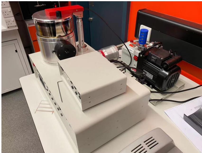
Figure 30 Desktop sputtering system used for the deposition of metal for surface plasmonic experiments.
