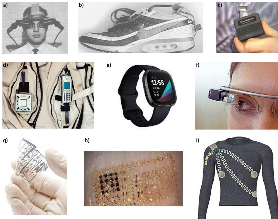
Figure 2.1 Wearable technology inventions including: a) the world's first head-mounted display 27 , b) the first wearable computer in shoe 28 , c) the active badge location system 29 ; commercial products such as: d) Levi's industrial clothing division jacket, e) Fitbit f) Google Glass; prototypes of: printed flexible electronics on plastic films g) 30 , skins h) 31 , and textiles i) 32 .
