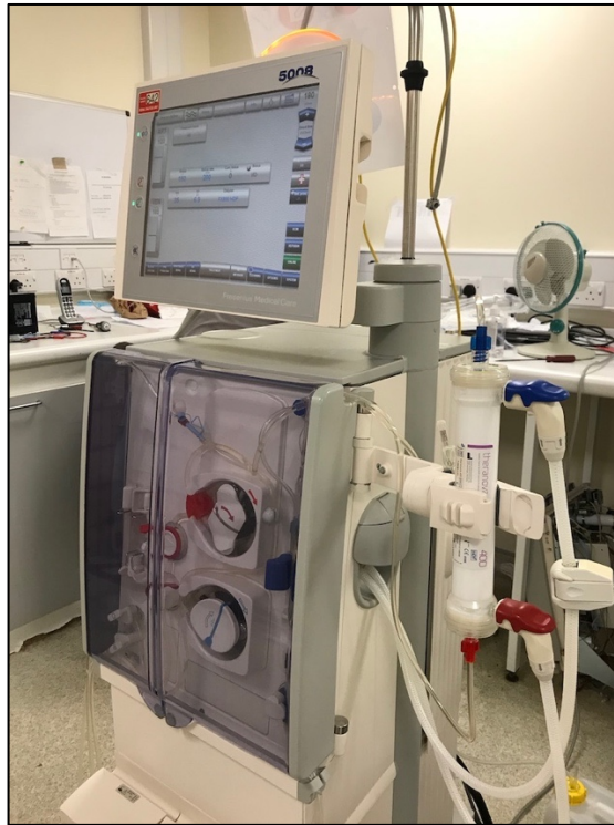
Image8-5: Fresenius 5008® device used in the study. Setup shown with the MCO dialyser connected. The same machine was also used for HDF treatment.
