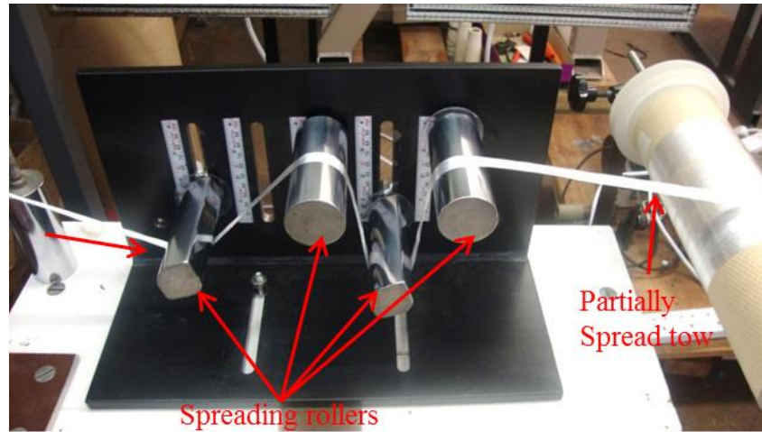
Figure 3.5: Photograph of roller spreading process.
