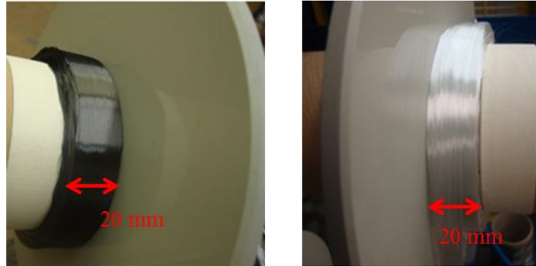
Figure 3.7: Spread tows (a) 12 K carbon fibre and (b) 2400 tex E-glass fibre.
