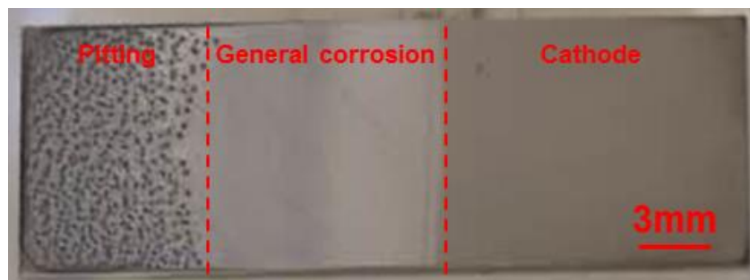
Figure 6.4- 2 Appearance of the BPE after the bipolar experiment after 30 min. exposure.
