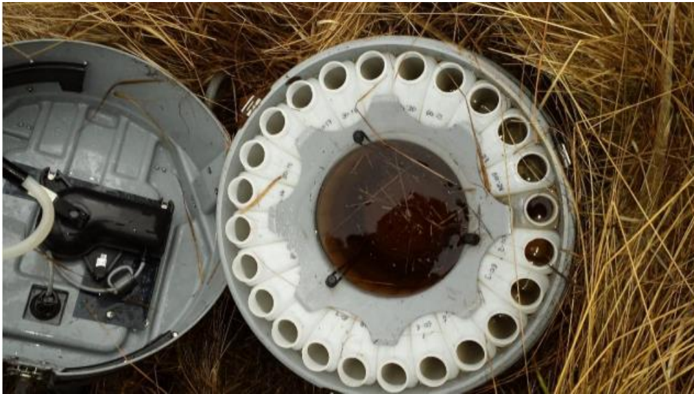
Figure 9 Sigma SD900 auto sampler with collected samples.
