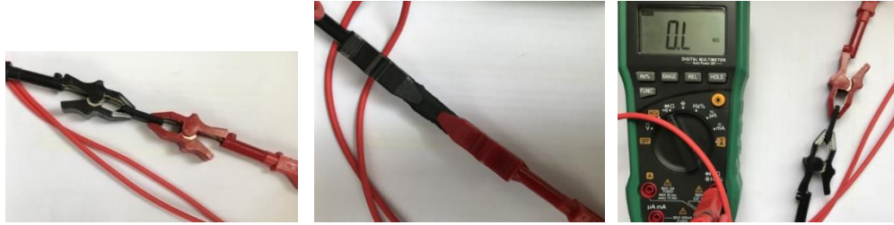
Figure 4-21: Placement of resistance measurement terminals using the 600V AC/DC multi-meter.
