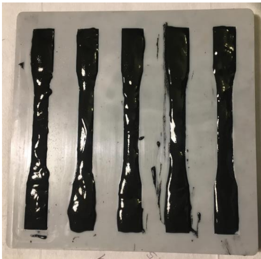
Stage 3: Layup of samples, and comparison of on the left using high temperatures, whilst on the right using SG with low temperatures.
