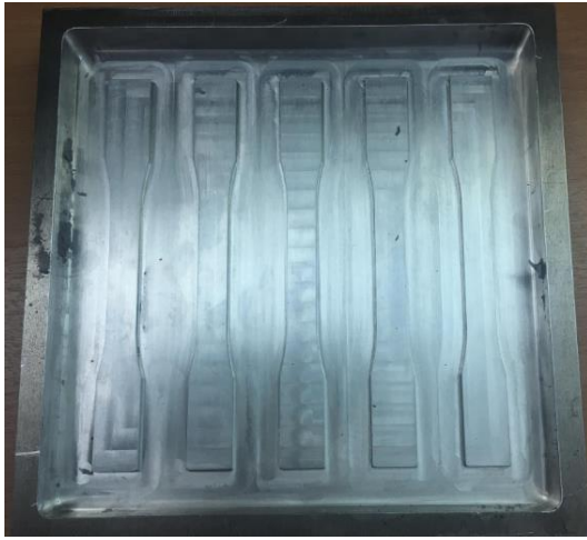
Stage 1: Negative metal cast, tool making mould.
