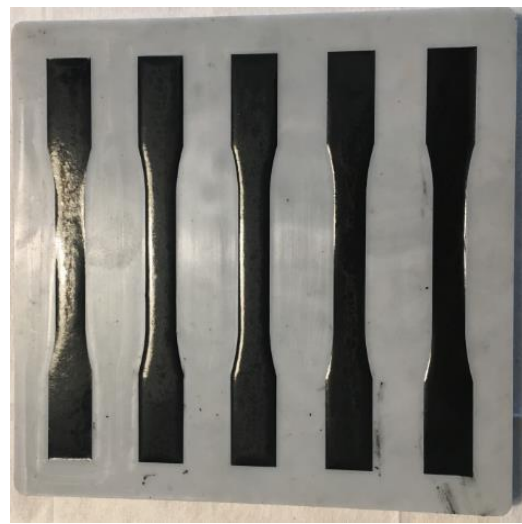
Stage 3: Layup of samples, and comparison of on the left using high temperatures, whilst on the right using SG with low temperatures.
