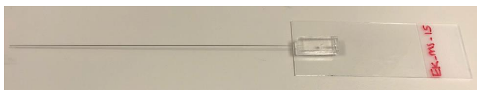
Figure 6.4.3: Droplet generation microfluidic chip with mass spectrometry emitter outlet.
