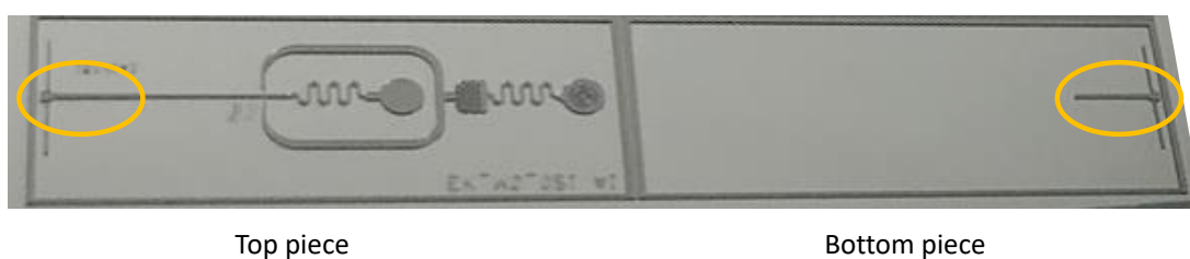
Figure 6.3.17: Example of a double layer mass spectrometry chip design. The pieces that will form the top and bottom of the PDMS chip are as indicated. The areas highlighted with the orange rings require alignment during the assembly of the top and bottom PDMS pieces.
