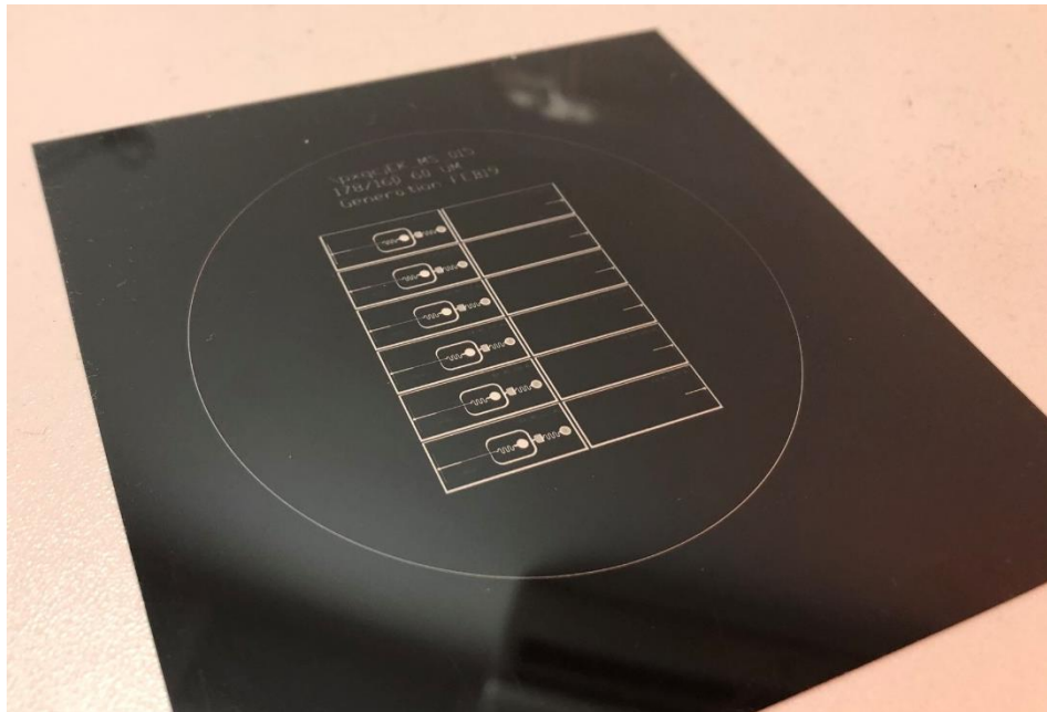
Figure 6.3.7: Photograph of a photolithography film mask received from Micro Lithography Services Ltd and cut to size (~10 cm by 10 cm) for use in subsequent fabrication steps.
