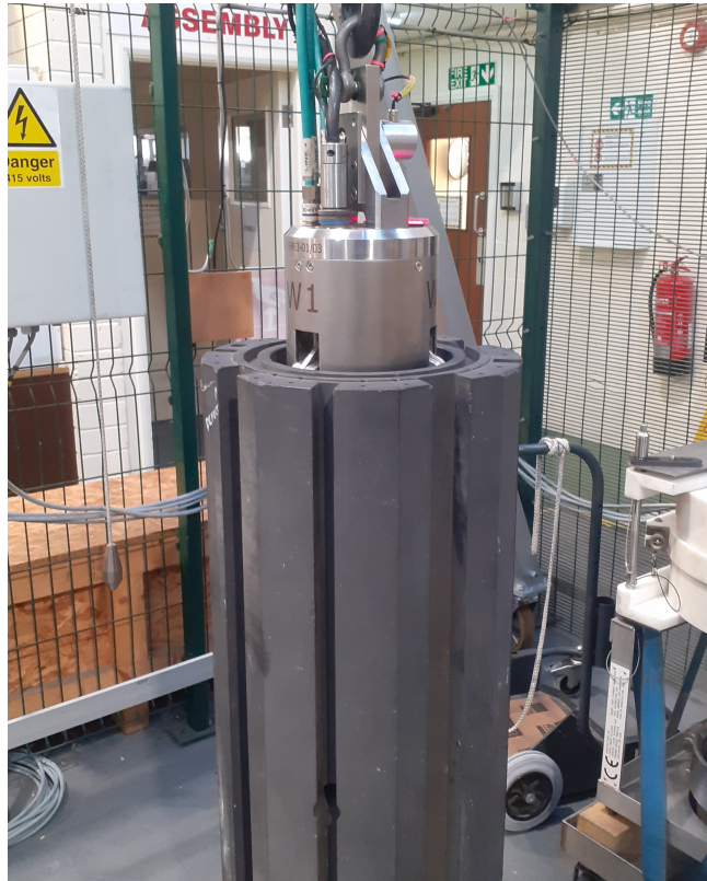
Figure 1: The application considered in this paper: the eddy current inspection of the nuclear moderator channels within advanced gas-cooled reactors.
