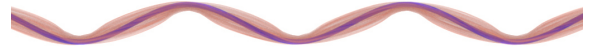
Fig. 10. Centerline of a fiber bundle. A yarn is simulated at fiber level with individual fibers shown in blue. The yarn’s centerline is highlighted in red. We fit yarn-level parameters so that the yarn curve resulting from yarn-level simulation closely matches the centerline from fiber-level simulation.
