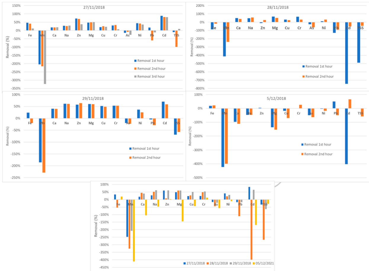
Figure 6. Removal of elements from Derriford SuDS1.
