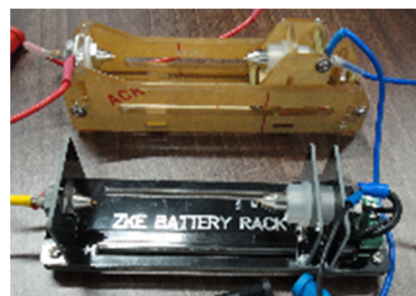
Figure 4. Spring loaded battery receptacles used in experimental research.
