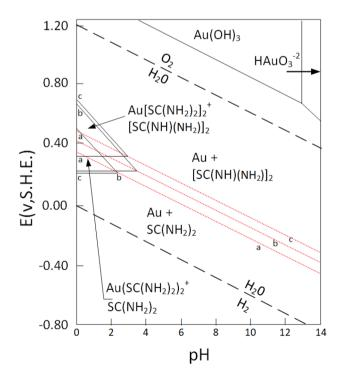
Fig. 1 Shows the Pourbaix diagram of the gold-thiourea complex in a  $H_2O_2$  system [60]
