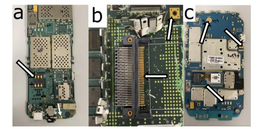
Fig. 2 Printed Circuit Boards. Gold location is indicated by white arrows; **a** Nokia 3310 PCB, **b** System X telecom PCB, **c** Blackberry PCB
