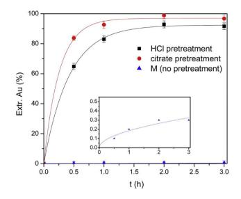
**Fig. 4** Gold leaching using thiourea (0.4 M thiourea, pH 1.5, 3 h) following pretreatment using HCl and Citrate and no pretreatment, M. Reprinted with perimission from [66]
