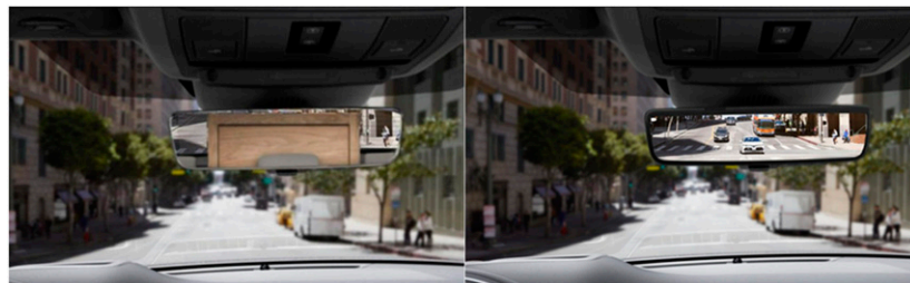
Figure 2. Traditional rear view mirror with rear view obscured by luggage (left image), versus the camera-based Clear View mirror (showing an enhanced view to the rear of the same car).
