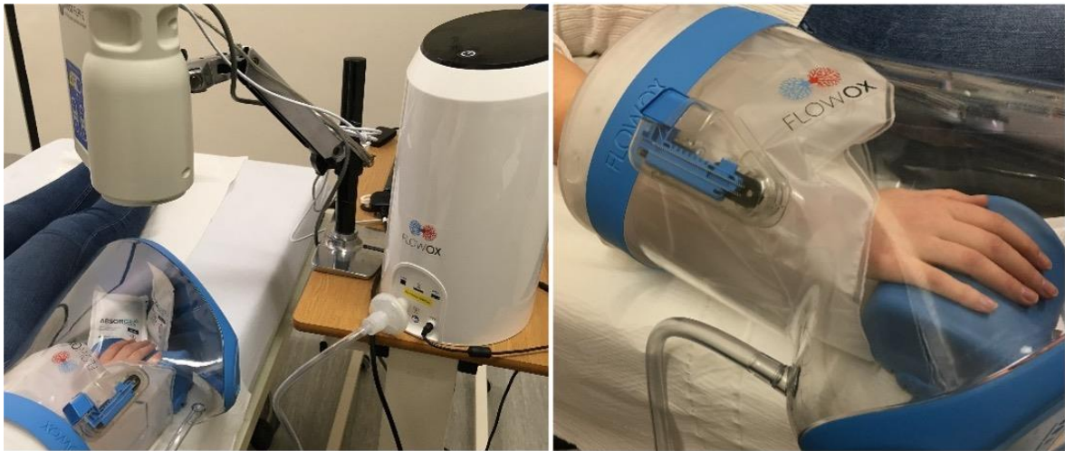
Figure 5.7 Full field laser speckle contrast imaging (FLPI) set up with Flow-Ox for assessment of blood perfusion in the hand. To assess blood perfusion of the dorsum of the hand and fingers while INP was applied, the participant's hand was placed inside the pressure chamber and rested on a hand rest. The FLPI imager was located at an appropriate distance from the surface of the hand and skin blood perfusion measured.
