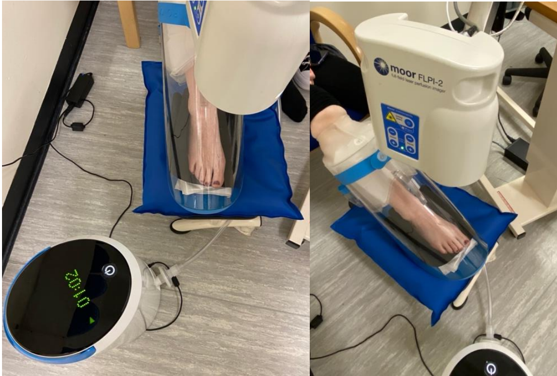
Figure 5.6 Full field laser speckle contrast imaging (FLPI) set up with Flow-Ox for assessment of blood perfusion in the foot. In order to assess blood perfusion of the dorsum of the foot while INP was applied, the participant's foot was placed inside the pressure chamber and rested on a footrest. The pressure chamber was rested on a small stool. The FLPI imager was located above the surface of the foot and skin blood perfusion measured.
