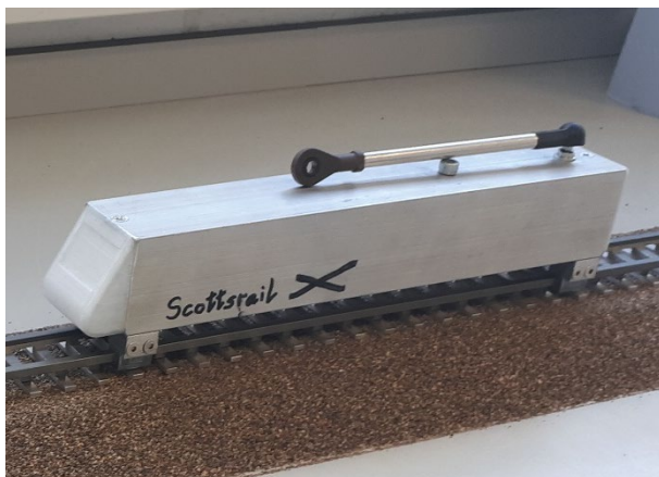
Figure 2. 1/50 th scale model train used to simulate a 68 tonne TGV-R power car (550 grams, 280 mm bogey spacing).
