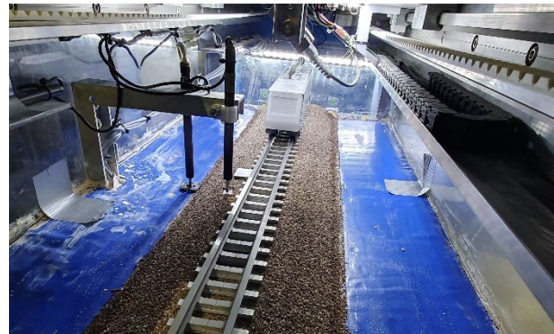
Figure 4. Model train and track on a model conventional ballasted embankment in the centrifuge actuation system.
