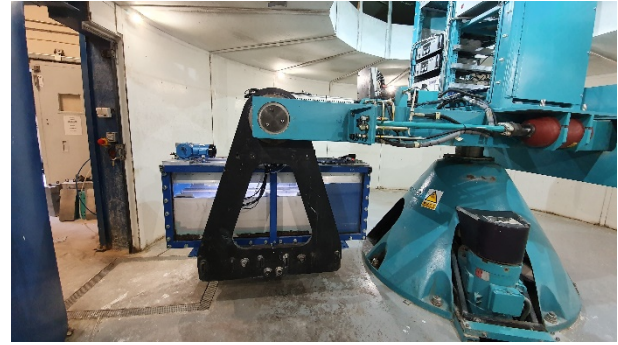
Figure 6. Rail simulator and 1.5 m long strong box installed on the University of Dundee's 3 m radius beam centrifuge.
