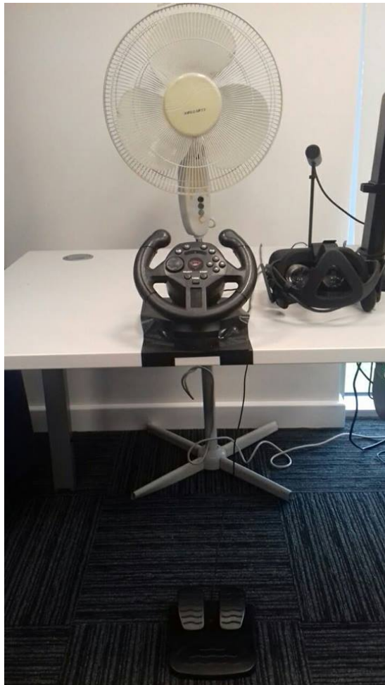
Figure 6.3: Study 2 Feedback Implementation: Visually unimpressive however gives a significant amount of feedback with noticeable variance based on virtual locomotion speed
