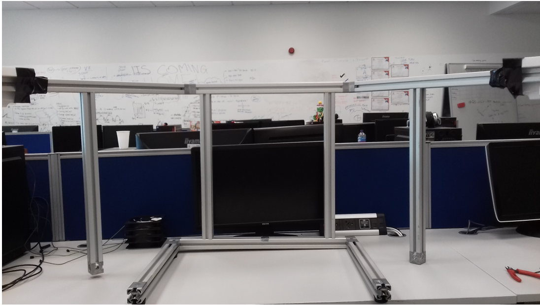
Figure 3.6: The extruded aluminium scaffolding used as a structure to mount airflow sources.
