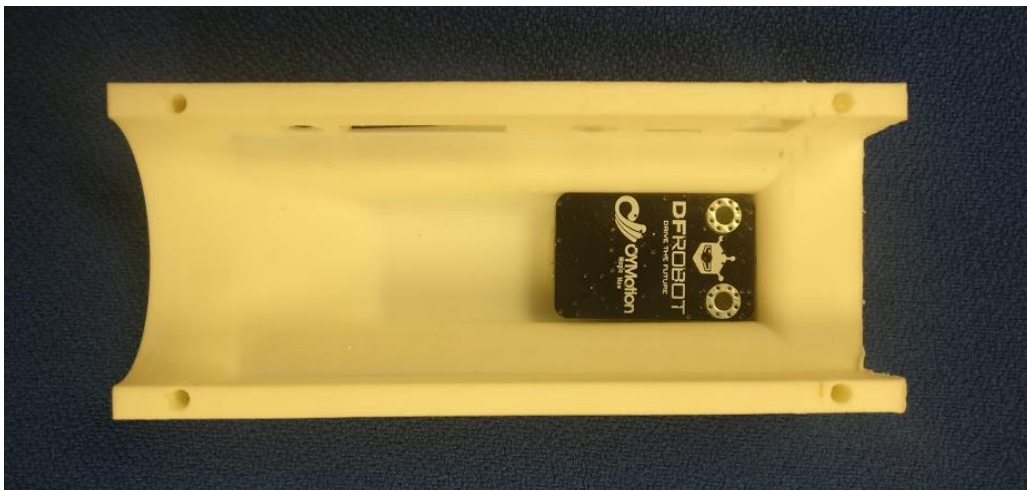
Figure 2.28 sEMG Filter Board Housing
