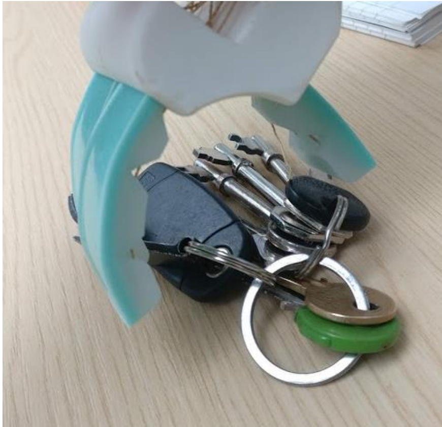
Figure 5.13 Attempted Grasp of 'Set of Keys' from a Flat Surface
