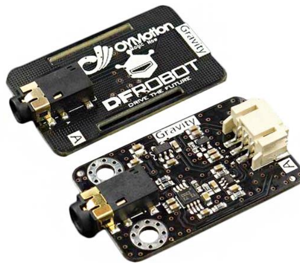
Figure 2.23 OYMotion Gravity: Analog EMG Sensor [96]
