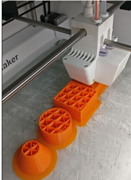
Figure 4.3 3D-Printing Process, Highlighting the Internal Structure
