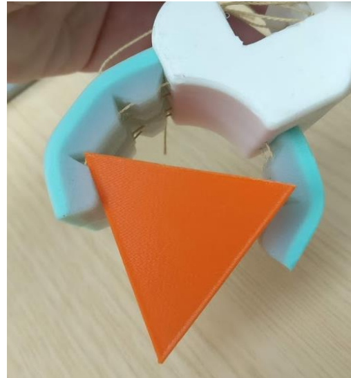
Figure 5.6 Pyramid under Successful Pinch Grasp
