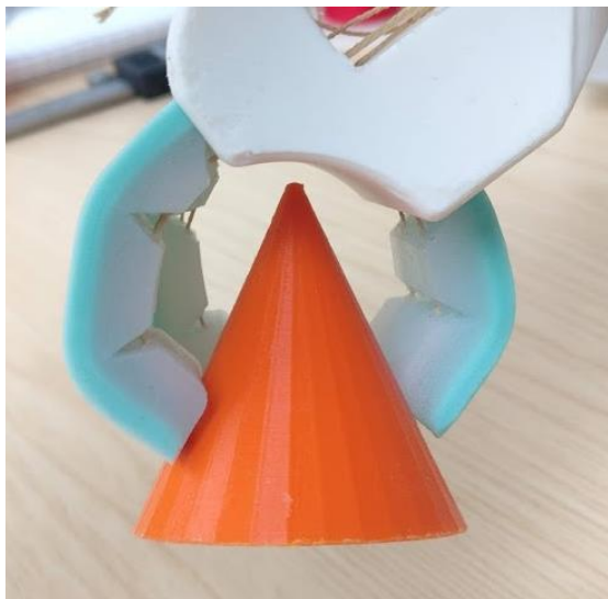
Figure 5.3 Cone under Failed Pinch Grasp
