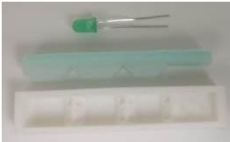
Figure 0.2 Mould, Soft Gripper, and 5mm LED for Scale
