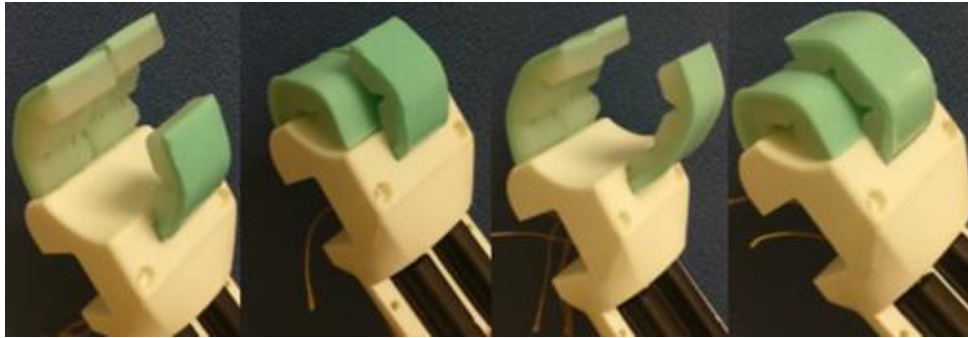
Figure 6.5 End Device in "Closed" and "Partly Open" Formations
