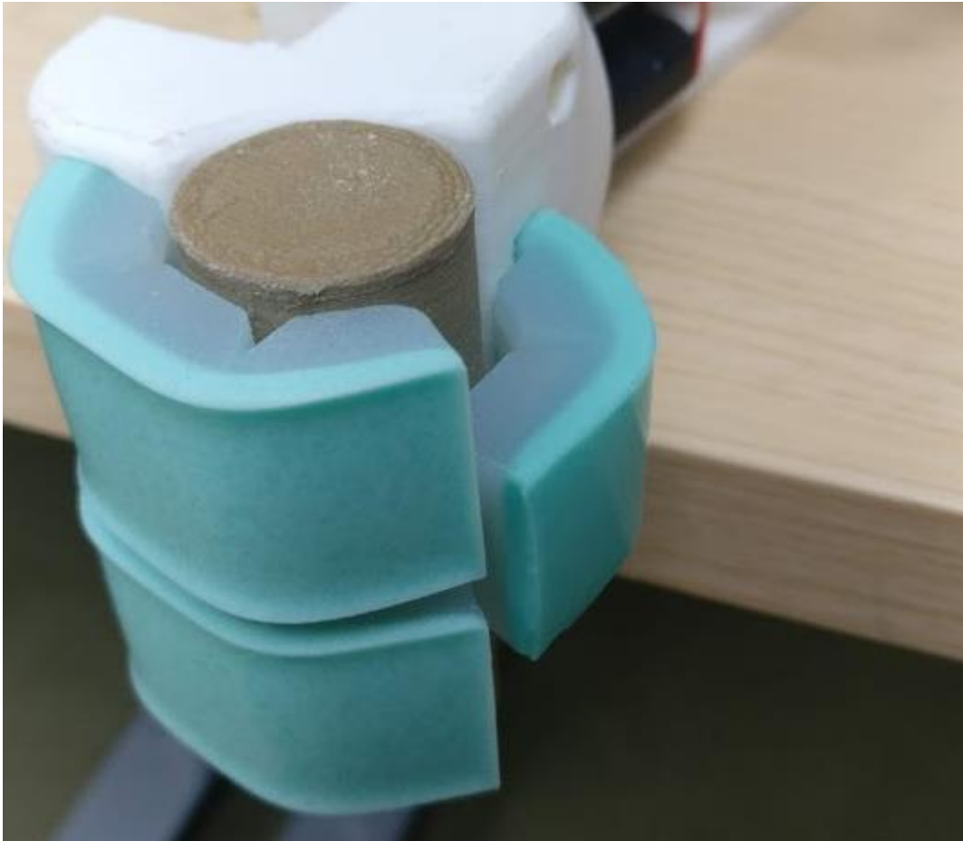
Figure 5.29 Grasp of 22.5mm Cylinder using 2-Segment Thumb
