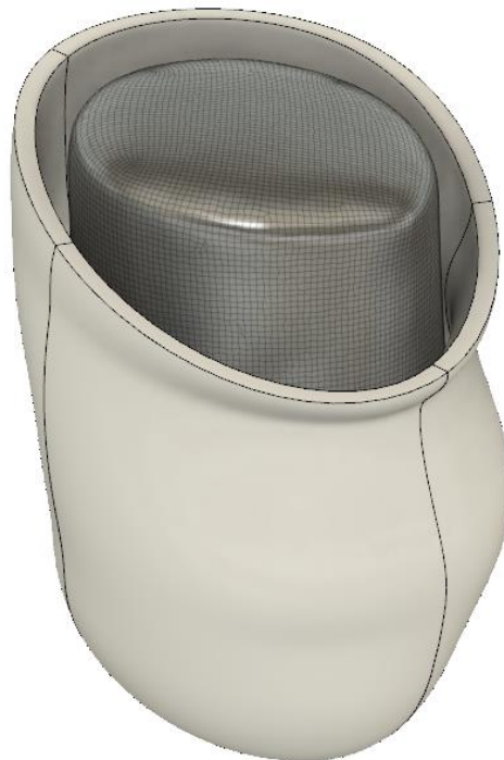
Figure 0.30 Socket with 3mm Wall thickness
