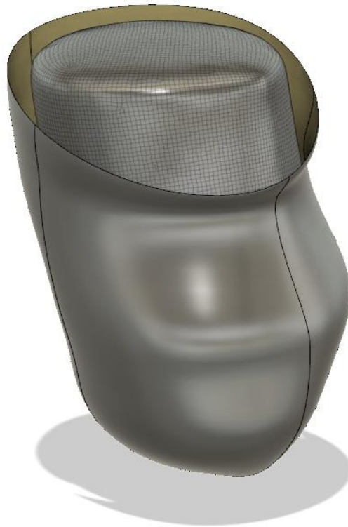
Figure 0.29 Socket Design in Solid Model Environment
