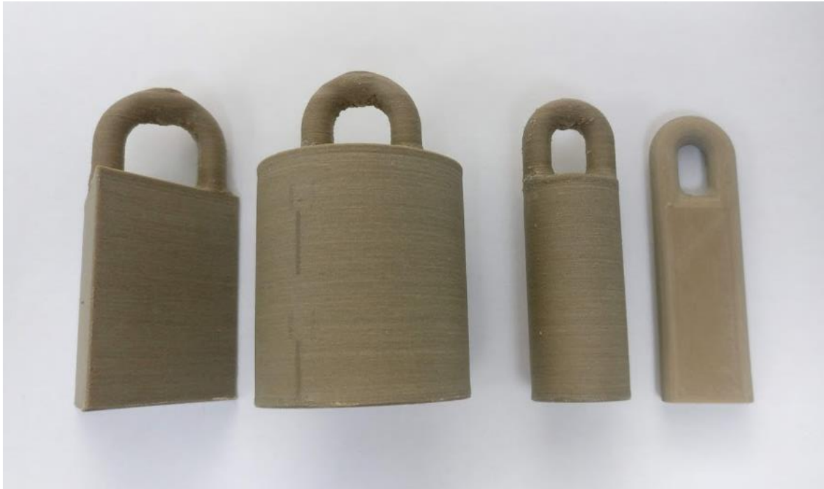
Figure 4.5 3D-Printed Objects for 'Weighted Test'
