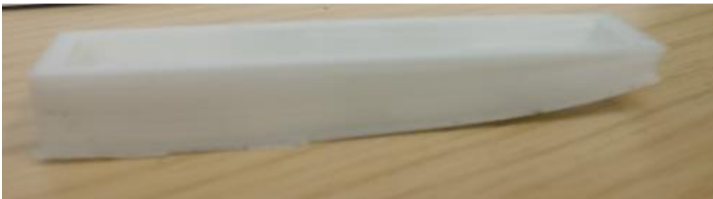
Figure 0.1 First Mould Print Displaying Warping
