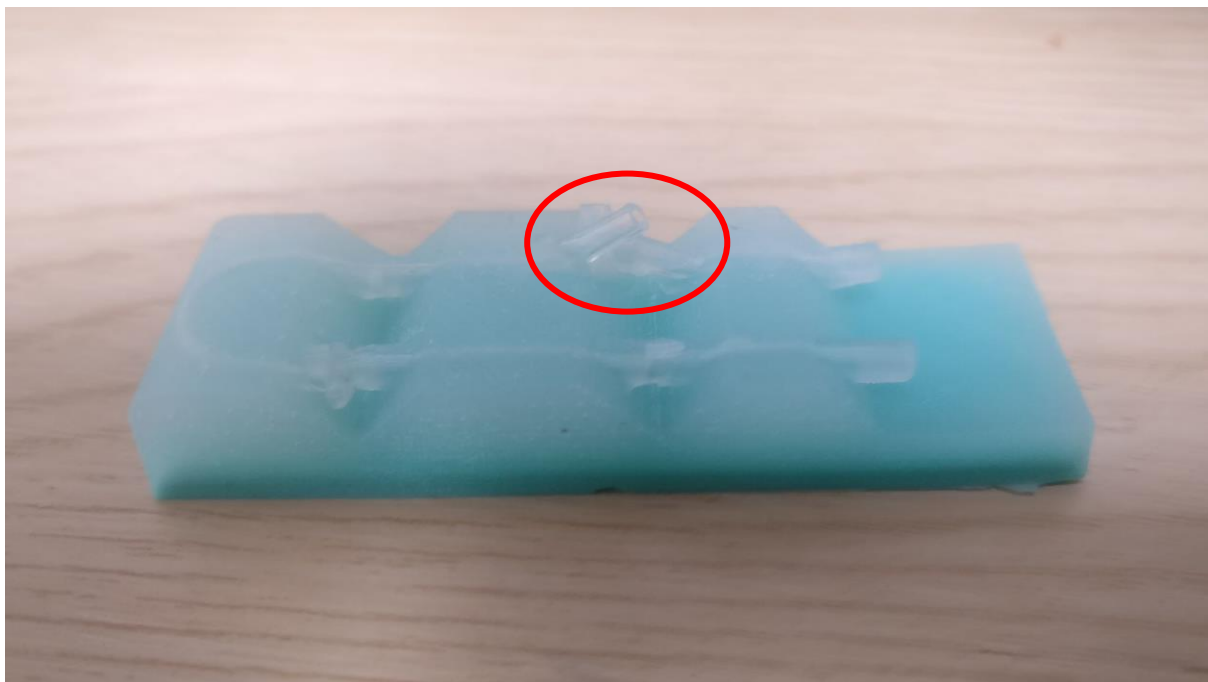
Figure 0.6 Soft-Gripper with Extruding Internal Tubes
