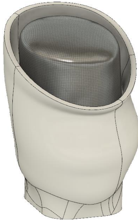
Figure 2.32 Socket with Attachment Structure
