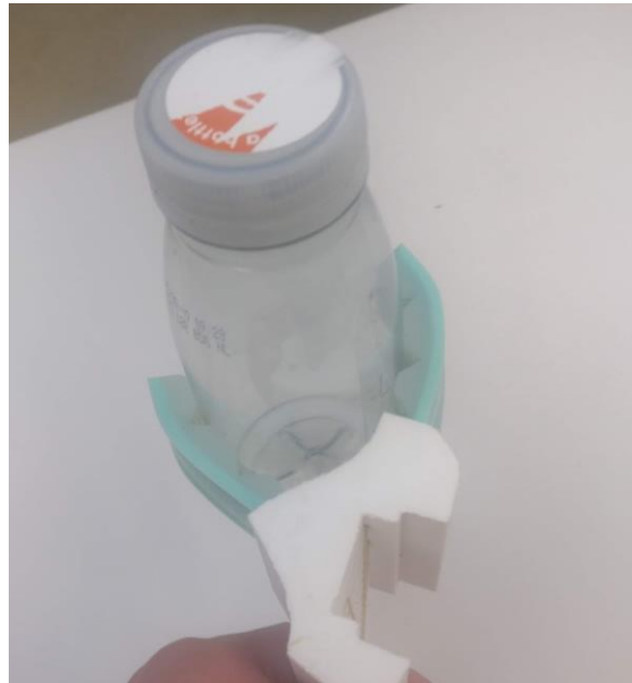
Figure 2.19 Prototype 45° Hand Grasping a Plastic Bottle
