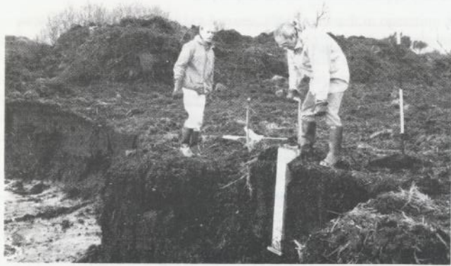
Figure 2. Mk 2 prototype peat cutter being used to sample raised mire peats at White Moss, Cheshire.
