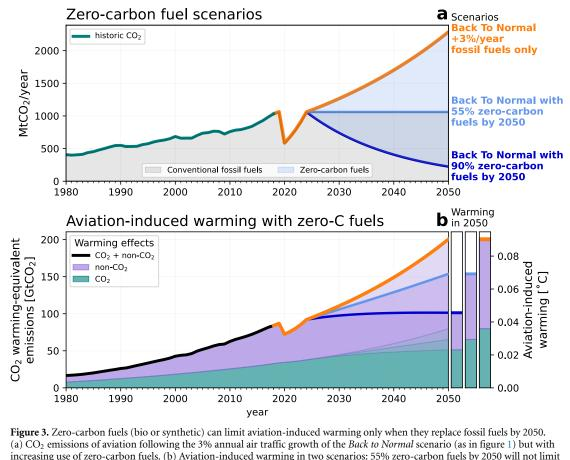
(a)  $CO_2$  emissions of aviation following the 3% annual air traffic growth of the *Back to Normal* scenario (as in figure 1) but with increasing use of zero-carbon fuels. (b) Aviation-induced warming in two scenarios: 55% zero-carbon fuels by 2050 will not limit the warming, only the highly ambitious scenario of 90% carbon neutrality reaches a maximum warming of about 0.04 °C. Scenarios are colour-coded as in (a).
