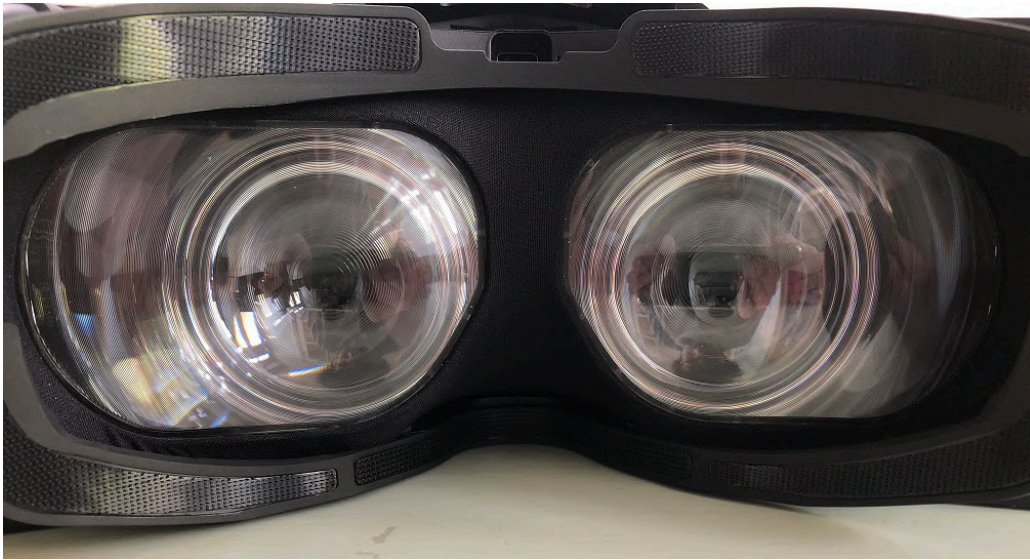
Figure 2.5: An example of the Pimax VR headset and its higher FoV lenses.
