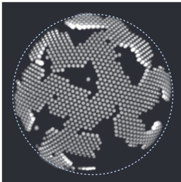
Figure 1.7: A spherical droplet formed in a water-in-oil system with radius 17.6 \mu\text{m} partially coated in particles. The droplets in the system encapsulate an aqueous mixture of 1.0 \mu\text{m} polystyrene (PS) spheres and 80 \text{ nm} poly( N -isopropylacrylamide) [poly(NIPAM)] particles. Ribbon-like crystals can be seen on the surface. From work by Meng et al. 81
