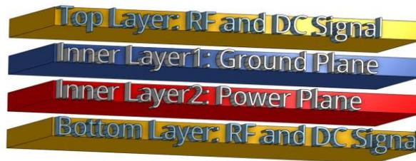
Figure 7.12: Four-layer PCB stack.
