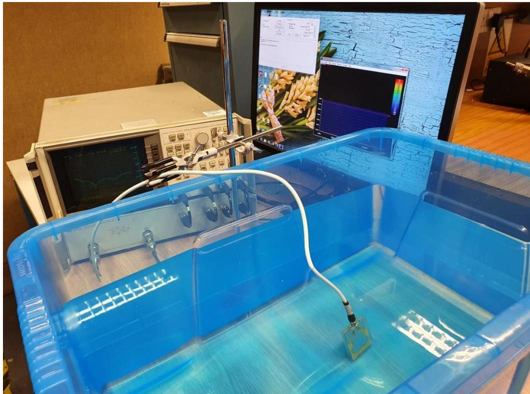
Figure 4.32: Experimental setup for underwater antenna tests.
