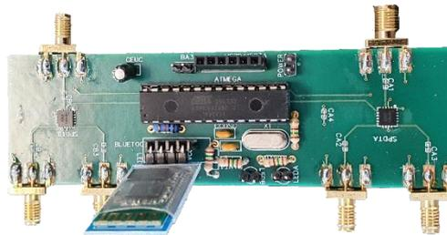
Figure 7.17: PCB controller for oil slick thickness measurement.
