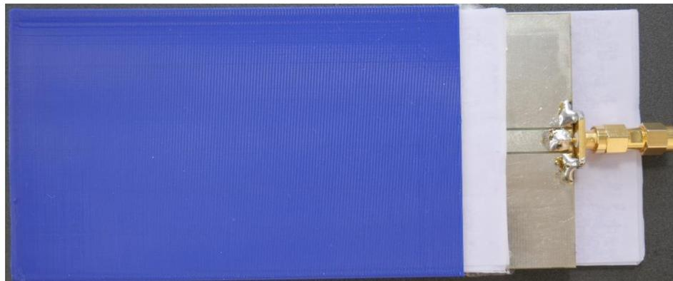
Figure 6.13: Oil-treated papers, barrier and braid antenna.
