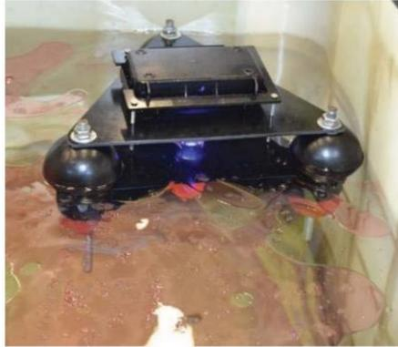
Figure 2.8: Led-based spectrometer sensor in tank with diesel film [31].
