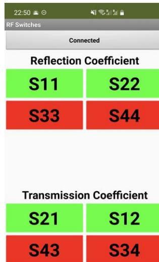
Figure 7.5: Android App for controlling and selecting RF switches.
