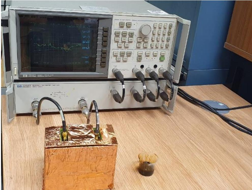
Figure 5.7: Experimental setup for the oil spill test for crude oil.
