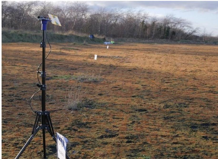
Figure 6.17: Setup for the received signal strength indicator (RSSI) tests for receive and transmit antennas.
