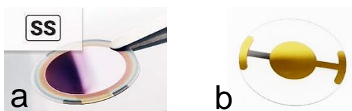
Figure 3.3. Surfaces of reference: (a) stainless steel and (b) gold sensors. Sensors have a diameter of 14 mm and a thickness of ca. 300 \mu\text{m} .
