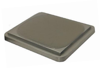
Figure 3.4. WPC fouled 316L stainless steel coupon. Dimensions of the coupon are detailed in section 3.2.1.
