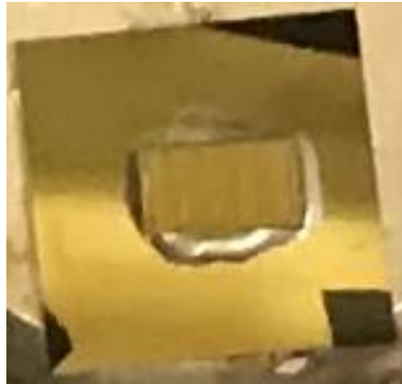
Figure 4. 8 Combination of the diamond heat spreader with GaN
