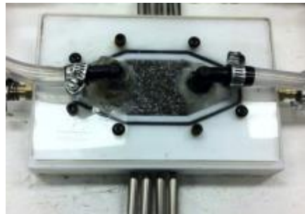
Figure 2. 13 A figure of metal foam based cooling channel [164]
