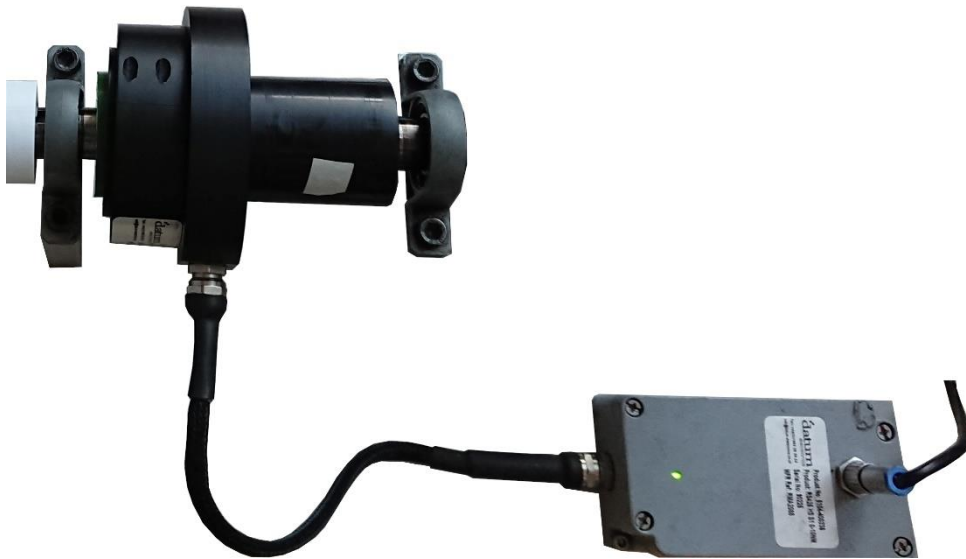
Figure 6.6 – Datum torque meter with signal conditioner
