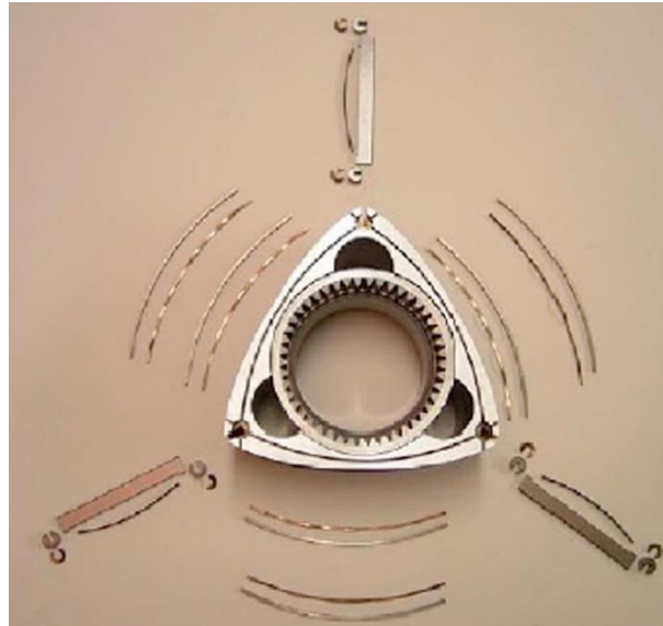
Figure 2.20 - Seals for a Wankel expander prototype [89]
