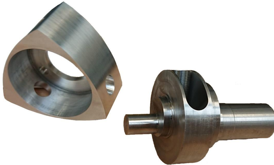
Figure 7.24 – Second prototype rotor (Aluminium 7075) and internal shaft (Steel)
