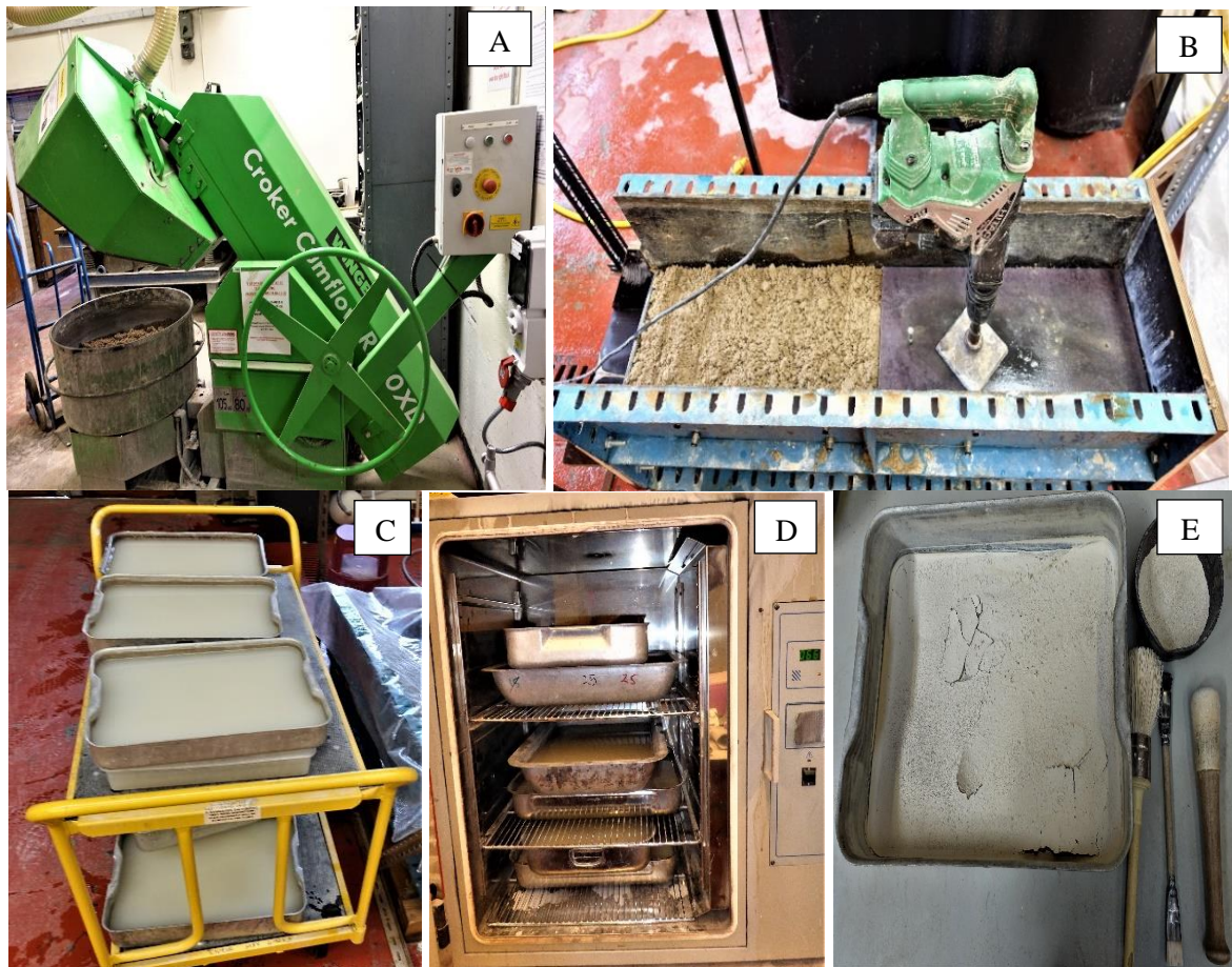
Figure 3. 16. Mixing samples in electric mixer (A); compaction by electric hammer (B); collected runoff and sediment (C); oven-drying sediment (D); and sediment for sieving (E)
