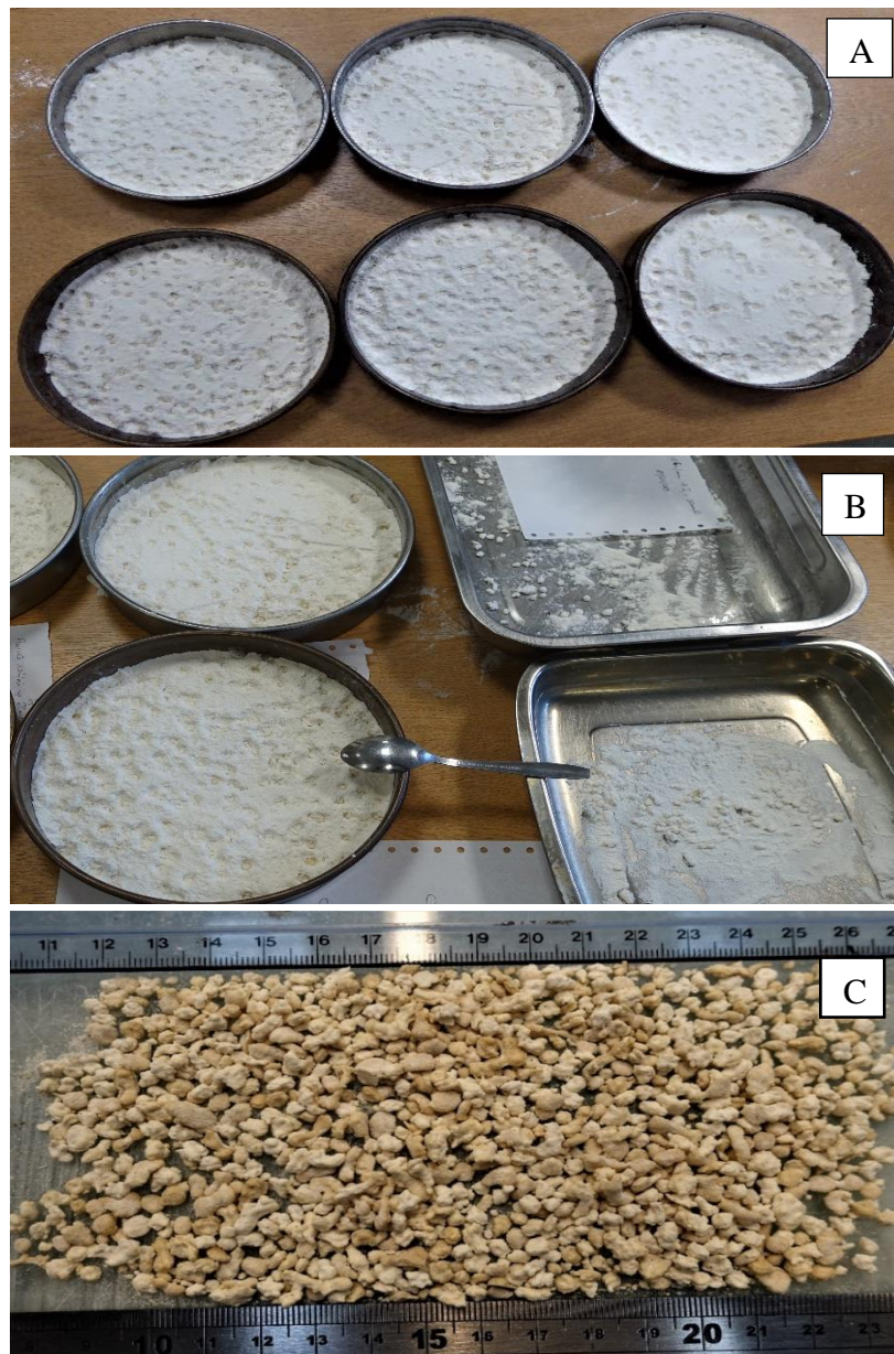
Figure 3. 10. Raindrops collection into the flour (A), separating air-dried pellets from the flour (B) and sieved oven-dried pellets (C)
