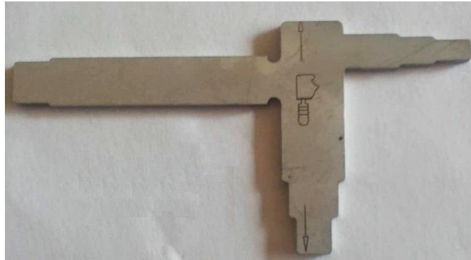
Figure 26: A Straumann diagnostic T Tool which can be used to gauge whether there is adequate intra-oral access to prepare the implant bed and place the dental implant.
