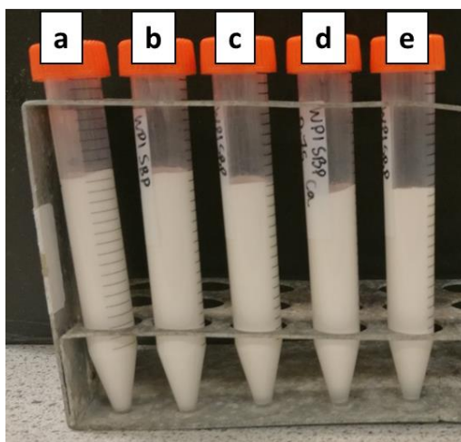
Figure 4-5: Photographs of centrifugation tubes containing 2.5% w/w WPI-SBP stabilised oil-in-water emulsions (20% w/w sunflower oil) with 1 mg.mL -1 (a), 2.5 mg.mL -1 (b), 5 mg.mL -1 (c), 7.5 mg.mL -1 (d) and 10 mg.mL -1 (e) CaCl 2 added before emulsification. Photographs were taken immediately after centrifugation.
