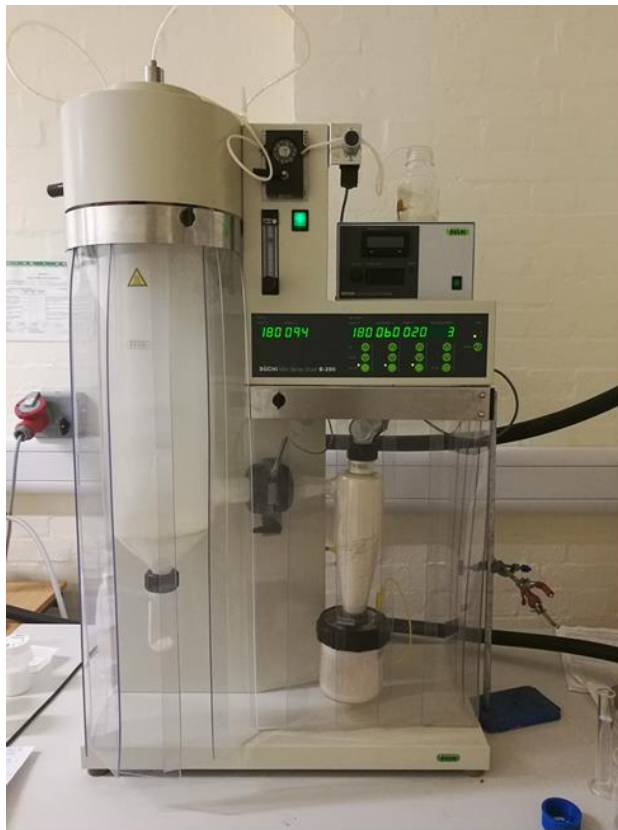
Figure 2-11: Photograph (left) of a Buchi Mini Spray Dryer B-290 (University of Birmingham) and schematic representation (right) of the spray drying process.
