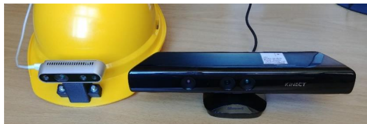
Figure 6-3: Intel RealSense D435 mounted onto a hard hat next to a Microsoft Kinect
