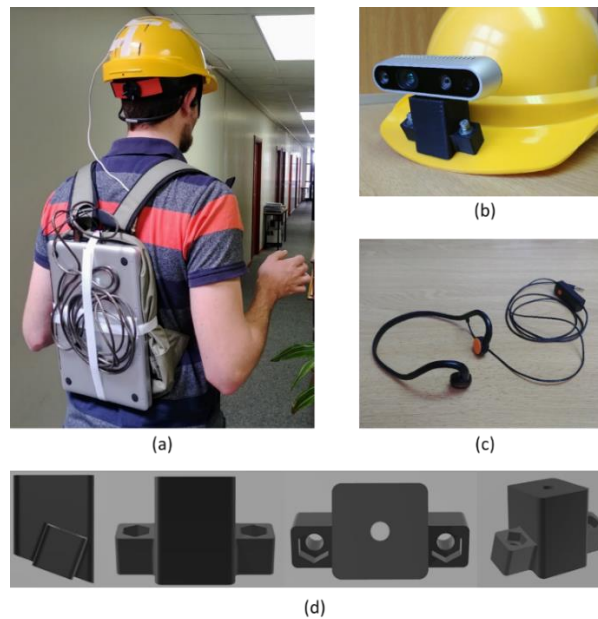
Figure 6-2: Hardware used for the prototype. The full sensory substitution system (a), a close-up of the depth camera mounted to a hard hat (b), a close-up of the bone conduction headphones (c), multiple angles of the 3D printed mount used to connect the depth camera to the hard hat (d).
