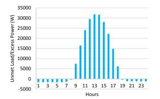
Fig. 7. Unmet load (negative values) and excess power (positive values) profiles
