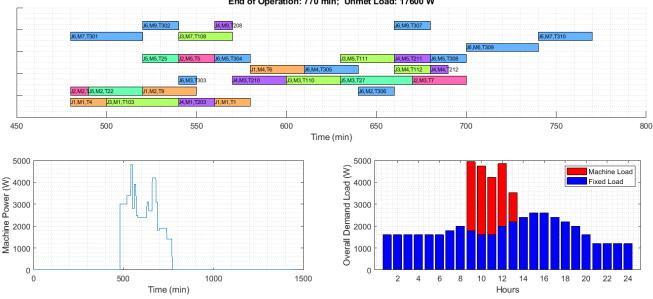
Optimum Solution w.r.t. Objective: Unmet Load End of Operation: 770 min; Unmet Load: 17600 W
