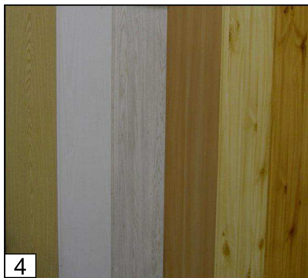
Pic. 4. Organic materials for finishing interior walls and ceilings: 1,2 – wallpaper; 3 – acoustic board from polymer materials; 4 – decorative veneer; 5 – panels from polymer materials.
