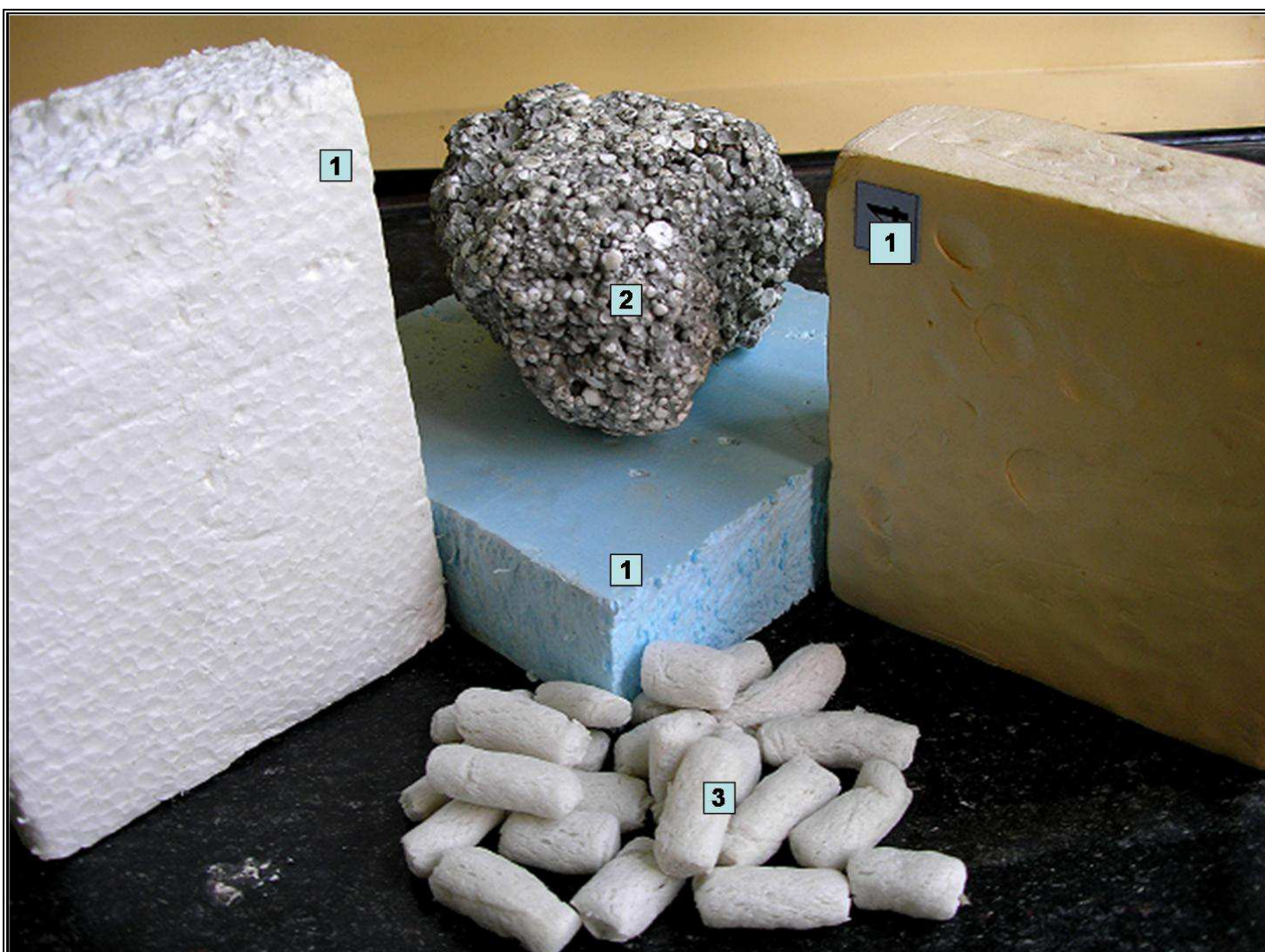
Pic. 6. Heat insulating materials on the basis of polymers: 1, 2 – slabs; 3 – granulated
