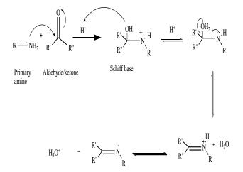
Scheme 2: General mechanism of formation of Schiff base
