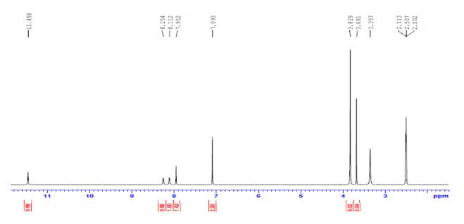
Fig. 3.<sup>1</sup>H-NMR spectrum of (*E*)-2-(3,4,5-trimethoxybenzylidene)hydrazinecarbothioamide
