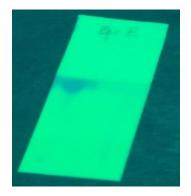
Fig. 1 TLC plate for (E)-2-(3,4,5-rimethoxybenzylidene)hydrazinecarbothioamide in ethanol as a eluent.
