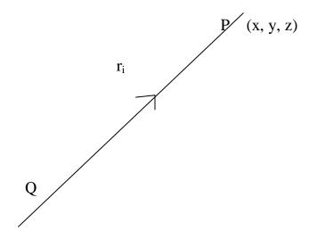
We define the electrostatic intensity or the electrostatic field vector at a point as the force that would act in vacuo on a unit charge placed at that point, due to the rest of the charges, provided the unit test charge is assumed not to disturb the field due to the other charges. This intensity has at each point a definite magnitude and a definite direction and is thus a vector. We denoted it by E. Thus for n charges
