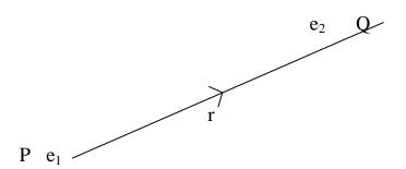
Where C is a constant and r is the position – vector of a relative to P. In C.G.S electrostatic unit system, we define a unit charge as one which, in vecuo, repels an exactly similar charge at a distance of one cm with a force of one dyne. In this system c = 1 and
