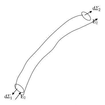
As there is no flux out of a tube of force, applying Gauss's theorem to the closed surface show in the figure.
