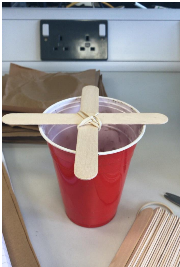
Figure 2.4: Wooden suspension apparatus used for decomposing the meat samples within water environments.
