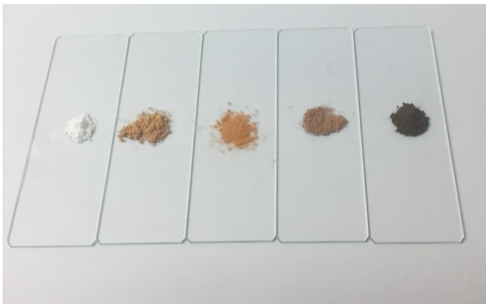
Figure 16 Photos of TiNT-catechol samples from left to the right: TiNT, TiNT-3,4-dihydroxybenzoic acid, TiNT-4-nitrocatechol, TiNT-3-hydroxytyrosol, and TiNT-dopamine. TiNT is white when the TiNT-catechol compounds show colours from light brown to dark brown.
