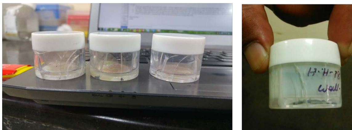
Figure 16: Cracked and opaque sample collection pots
