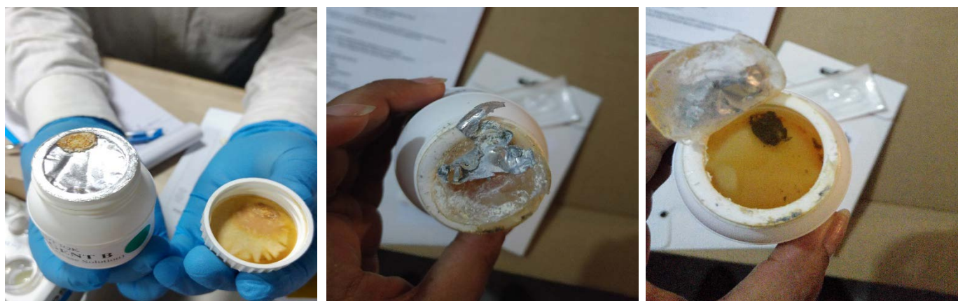
Figure 18: Images of reagent lids degraded and solution colour change
