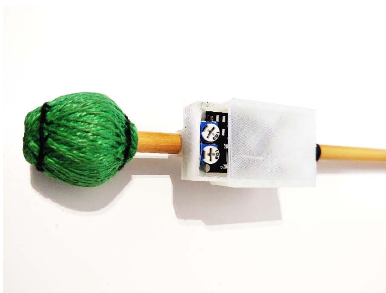
Figure 33. Immanence: Device #2 enclosed with 3D printed case and attached to a mallet.
