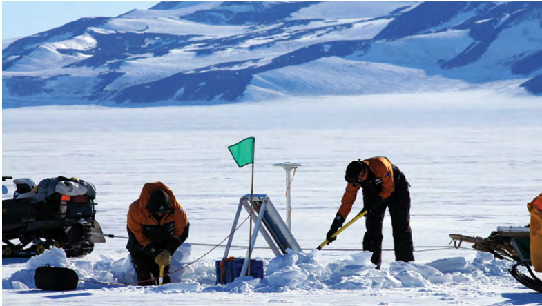
12.14 The solar power system used in the exhibition of Antarctic Sun Lines is shown here being used in Antarctic cryospheric fieldwork on the McMurdo Ice Shelf. Photograph by Wolfgang Rack, 2014.
