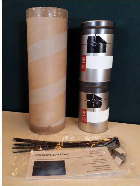
12.2 The package of pinhole cameras and installation instructions supplied to each Antarctic research station. Photograph by Adele Jackson, 2018.
