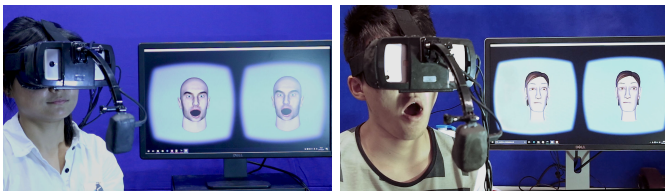
Fig. 17. A picture showing our system in action. Two users wearing HMDs are able to have immersive VR conversations even if they are at geographically distant locations. Their 3D face and eye gaze are captured and reconstructed in real time, and are then used to drive the animation of a 3D avatar shown on the VR display of the other subject in the conversation.
