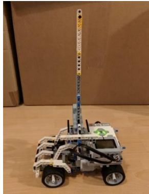
Figure 2.1: The single inverted pendulum on a cart (LEGO Mindstorms EV3)
