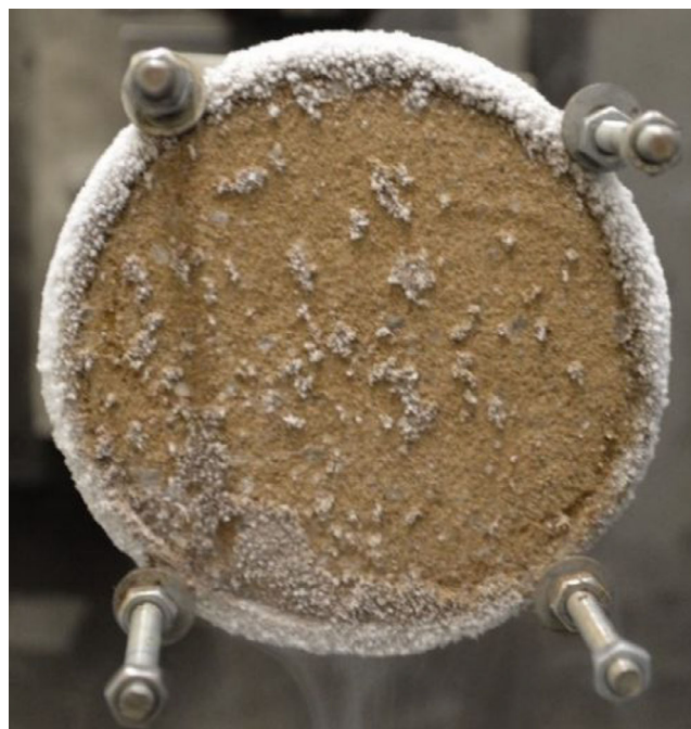
Fig. 1. A 100 mm diameter, stainless steel can containing a frozen ~50:50 mixture of finely crushed CO 2 ice and JSC-1 Martian regolith simulant. (Color figure can be viewed at wileyonlinelibrary.com .)
