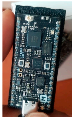
Figure 9. A nRF52840-MDK development kit used to configure the Thread network during the research [77].
