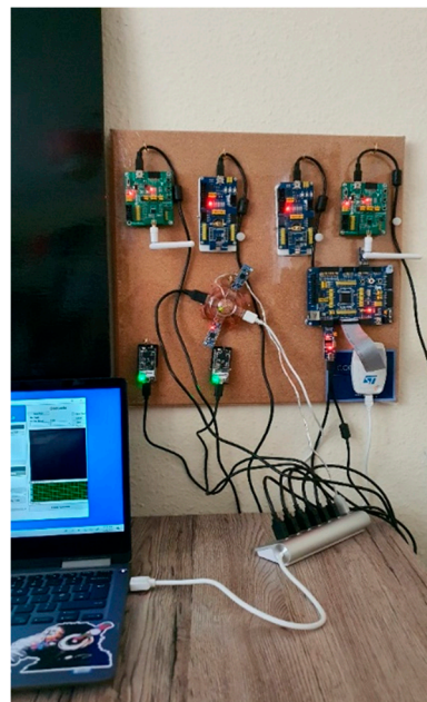
Figure 13. A JosNet Station Capable of Accommodating Multiple Network Technologies within a Single Station.
