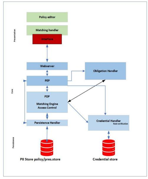
Figure 8: The PPL architecture (Curzon, et al. 2019, Enisa Europe 2019, Trabelsi, et al. 2011)
