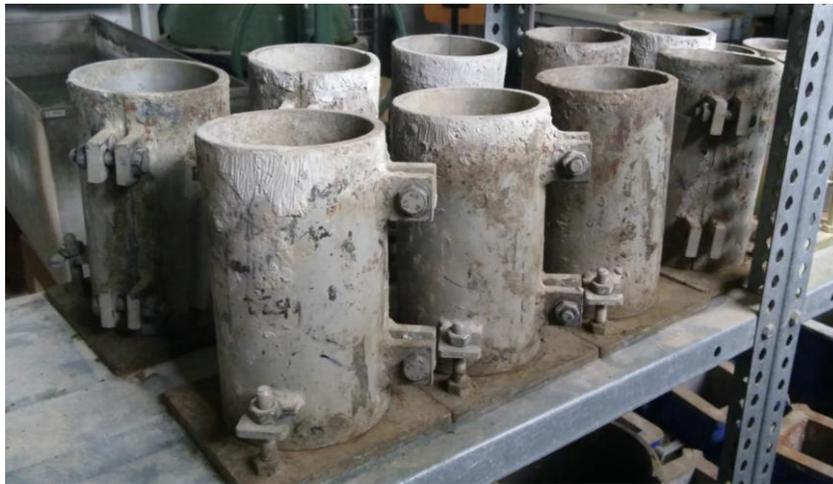
**Figura 20: Probetas de 100x200 mm**
