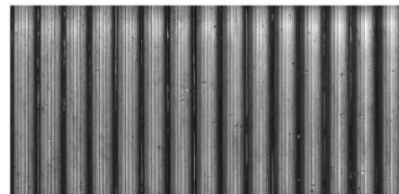
Figure 3. Original image with Ra 6.83 \mu\text{m} (low class).
