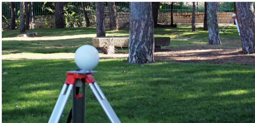
Figure 6. Reference network established for the study confirmed by spheres of 200 mm diameter.
