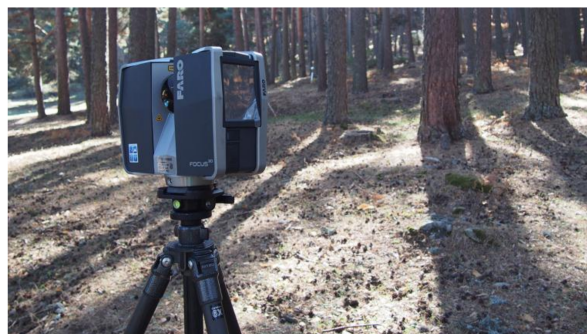
Figure 2. FARO Focus3D TLS device collecting 3D data in a forest environment.
