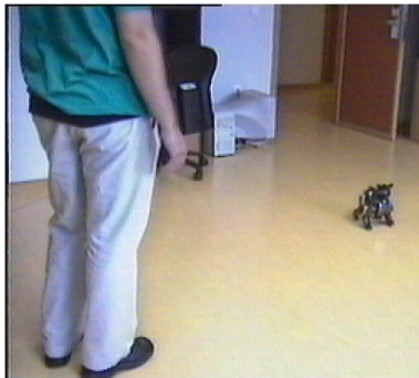
Figure 14: The robot spin if the distance is more than 1 meter and the angle if bigger than 50^\circ
