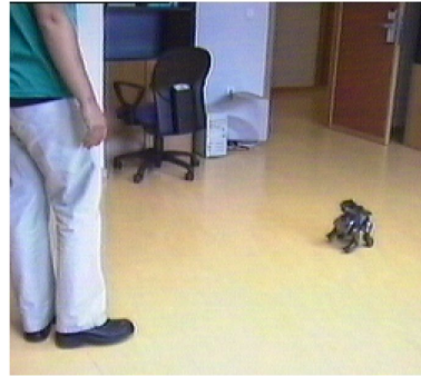
Figure 12: The robot goes forward if the distance is more than 1 meter and the angle is less than 10^\circ
