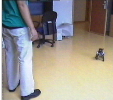
Figure 13: The robot spin and goes forward if the distance is more than 1 meter and the angle if between 10^\circ and 50^\circ
