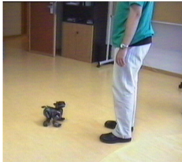
Figure 11: The robot stops if the distance is less than 1 meter
